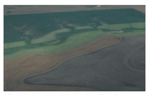
A filter strip helps keep sediment and farm chemicals out of this small stream.
